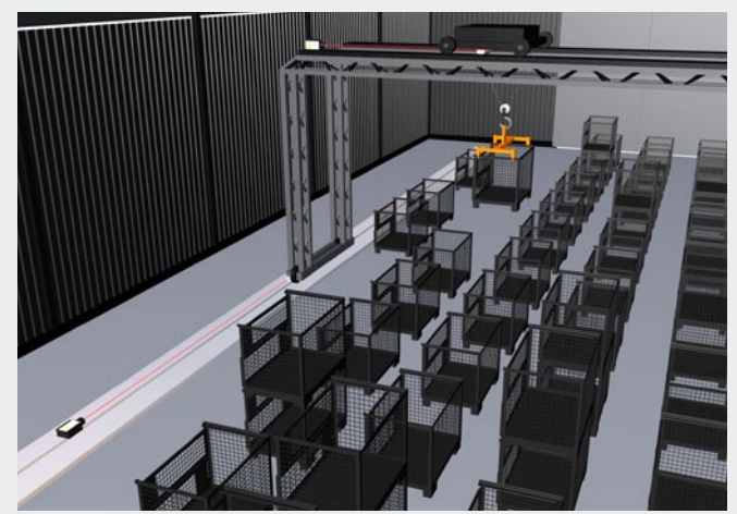
Position acquisition of gantry cranes and storage and retrieval units Fast response time in combination with high measurement accuracy facilitate the exact positioning of storage and retrieval units.
