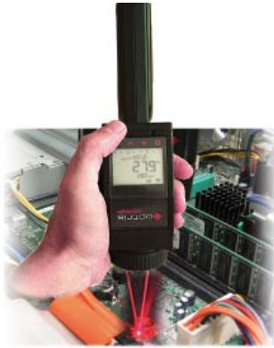
Highly accurate infrared temperature measurement with the optris LS of 1 mm small SMD components during a printed circuit board testing
